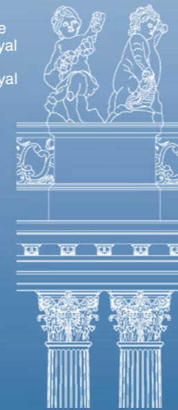
Detail drawing of Ringerkolonnade: capital, fascia and sculptures (fig.: STP, Bolze/Stich)
